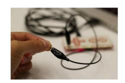
Connect to Arrows, Space, and Click —Connect one end of another alligator clip to arrow, space, or click on the board. Attach the other end to a conductive object.
