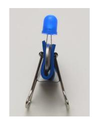
Use a binder clip, a battery, an LED, and foam to create a working circuit. Then make it interesting with craft materials!
